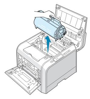
7 Take a new imaging unit out of the package using the handle.
